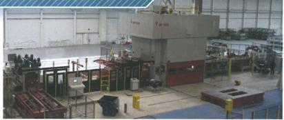
GONVAUTO Thuringen has ordered the supply, installation and commissioning of a new cutting line with blanking press to a consortium integrated by three Spanish companies: SALICO HISPANIA, ARISA and BIELE. The line is designed to cut blanks for the automotive sector, handling material of up to 3mm in thickness with maximum dimensions of 4500mm x 2500mm.
